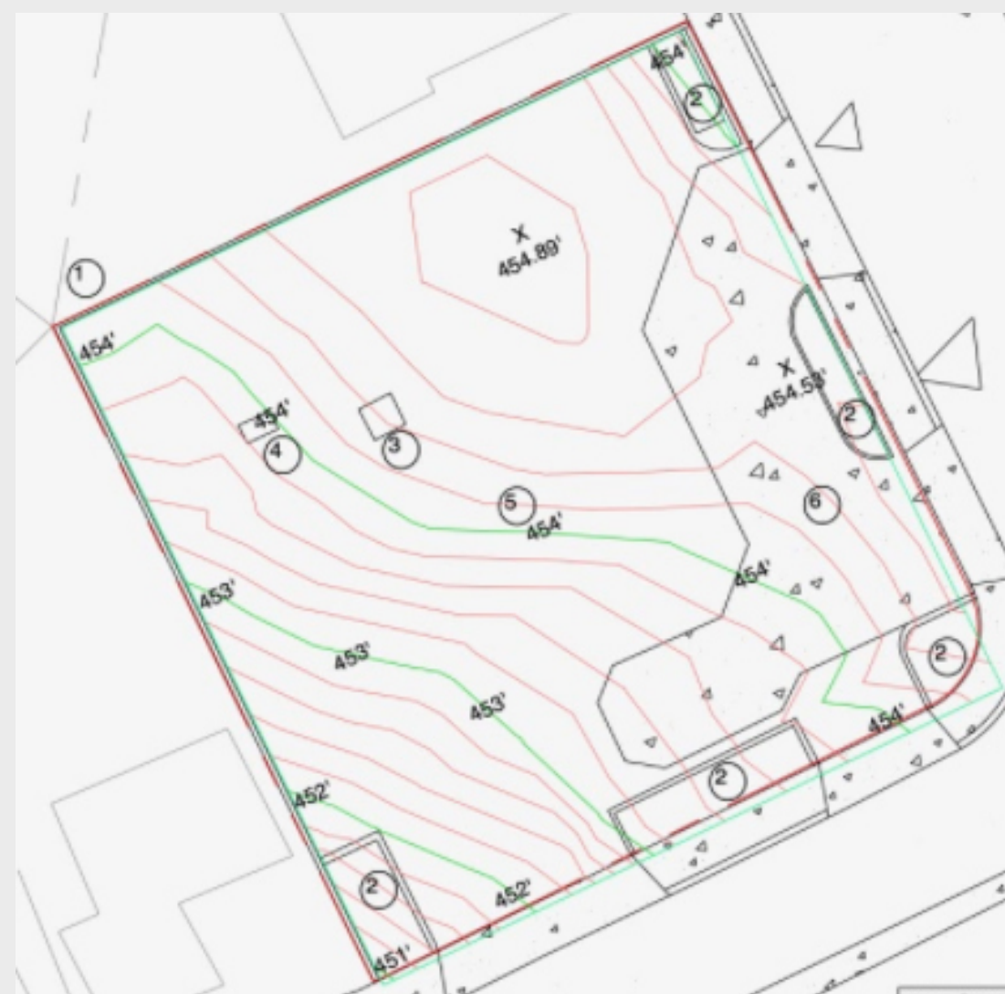
Site survey with marked elevations
