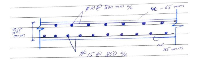
Deck slab reinforcement detail
